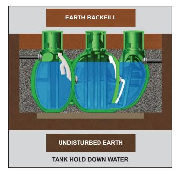
When pumping or dewatering the Singulair Green tank, only pump the pretreatment chamber. Then, promptly refill the tank to capacity with clean water. Dewatering and leaving the Singulair Green tank empty will effect tank integrity and void the Singulair Green warranty.
