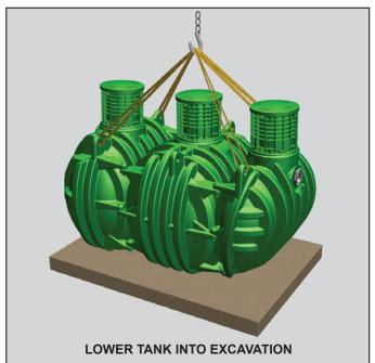
Remove the access covers and place a level on the risers to verify that the tank is level within 1/4" from side to side and end to end. If the tank needs to be raised more than 6" to apply leveling material, all personnel should move to a safe location so the tank can be fully removed from the excavation. Fall through the system from inlet invert to outlet invert is 4". Therefore, the outlet invert of the system
